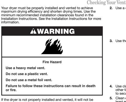
If the dryer is not properly installed and vented, it will not be covered under the warranty. Proper venting of your dryer is important for satisfactory drying results. See the Installation Instructions for more detail.
